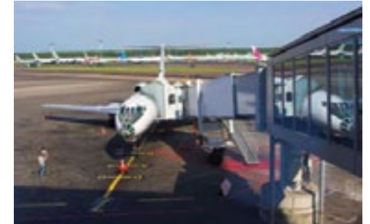
Laser range finding aircraft docking guidance systems with gate management software programs provide for accurate parking and bridge placement.
